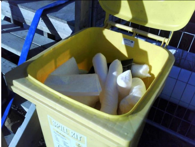
Photo 24 Spill kit better stocked. No list of contents or instructions in kit. Recommend that list and instructions be added to the kit.
