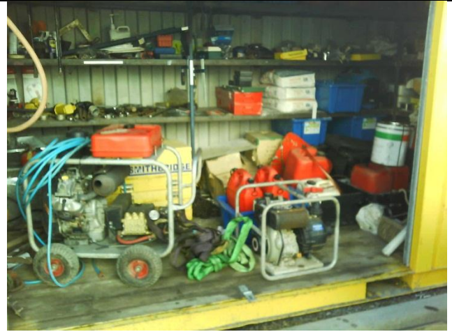
Photo 25 Example of acceptable storage of hazardous substances (plastic tubs used as secondary containment within unbanded container)
