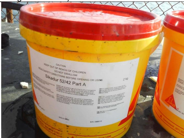
Photo 22 Further example of hazardous substances stored without secondary containment near water.
