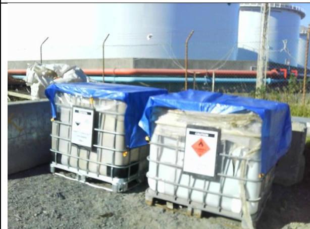
Photo 5 New waste bins for containers that have contained dangerous goods. Tarpaulin is used to keep out rain.
