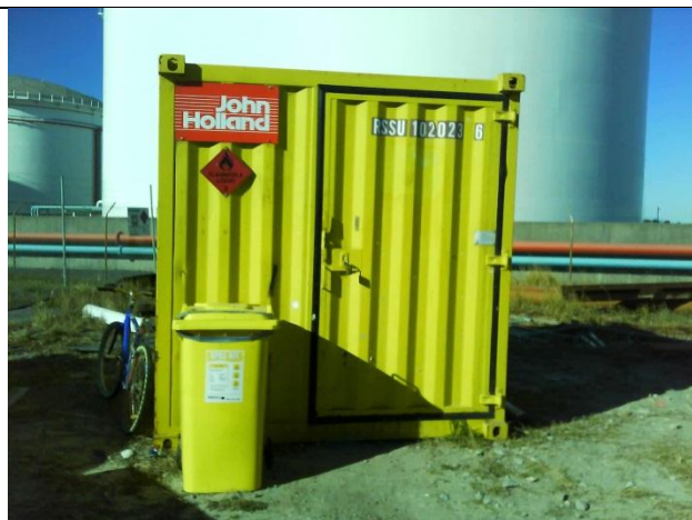
Photo 1 Hazardous substances storage container with spill kit (bunded)
