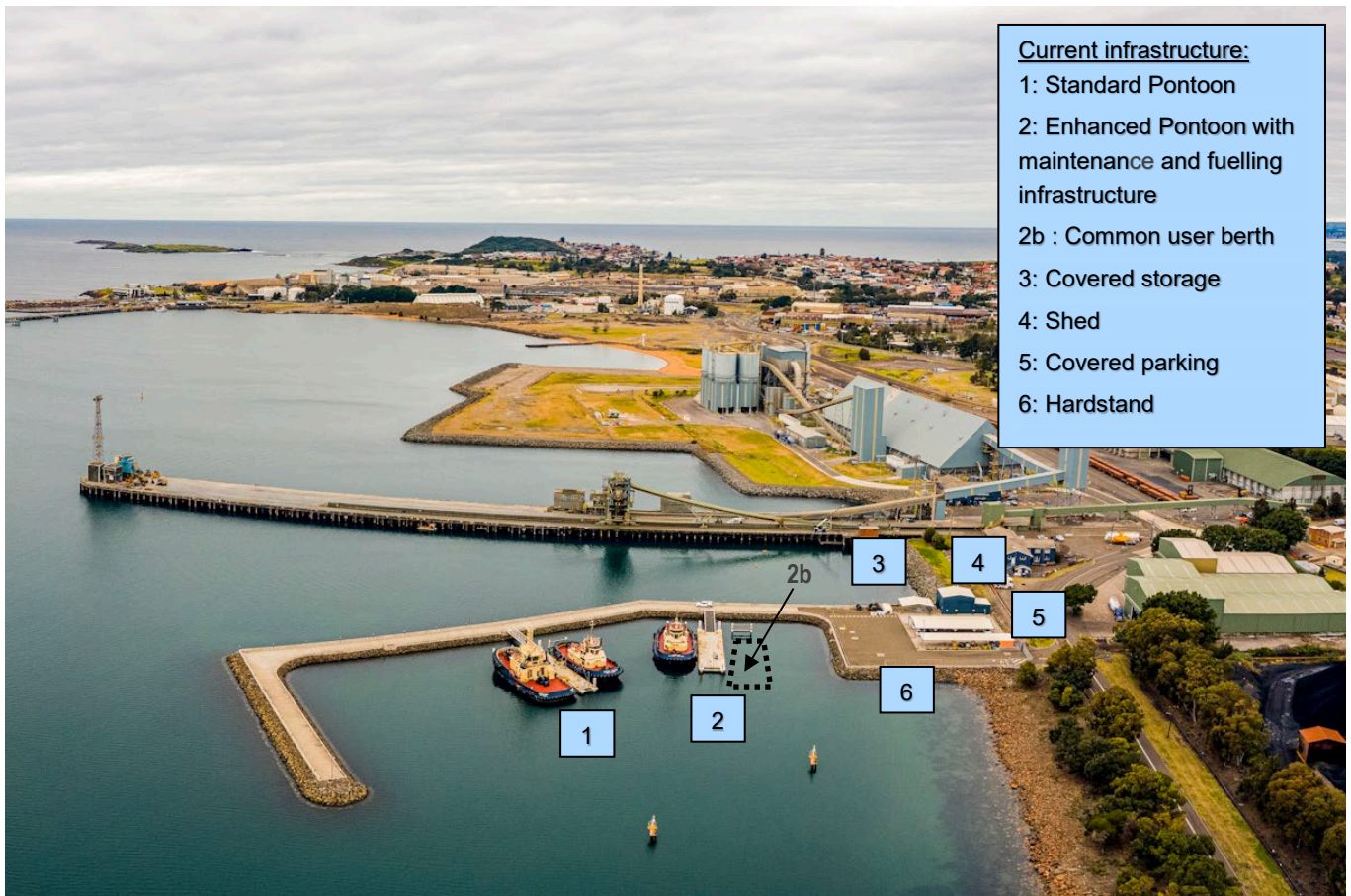
Diagram 1 – Location of existing waterside and landside Infrastructure
