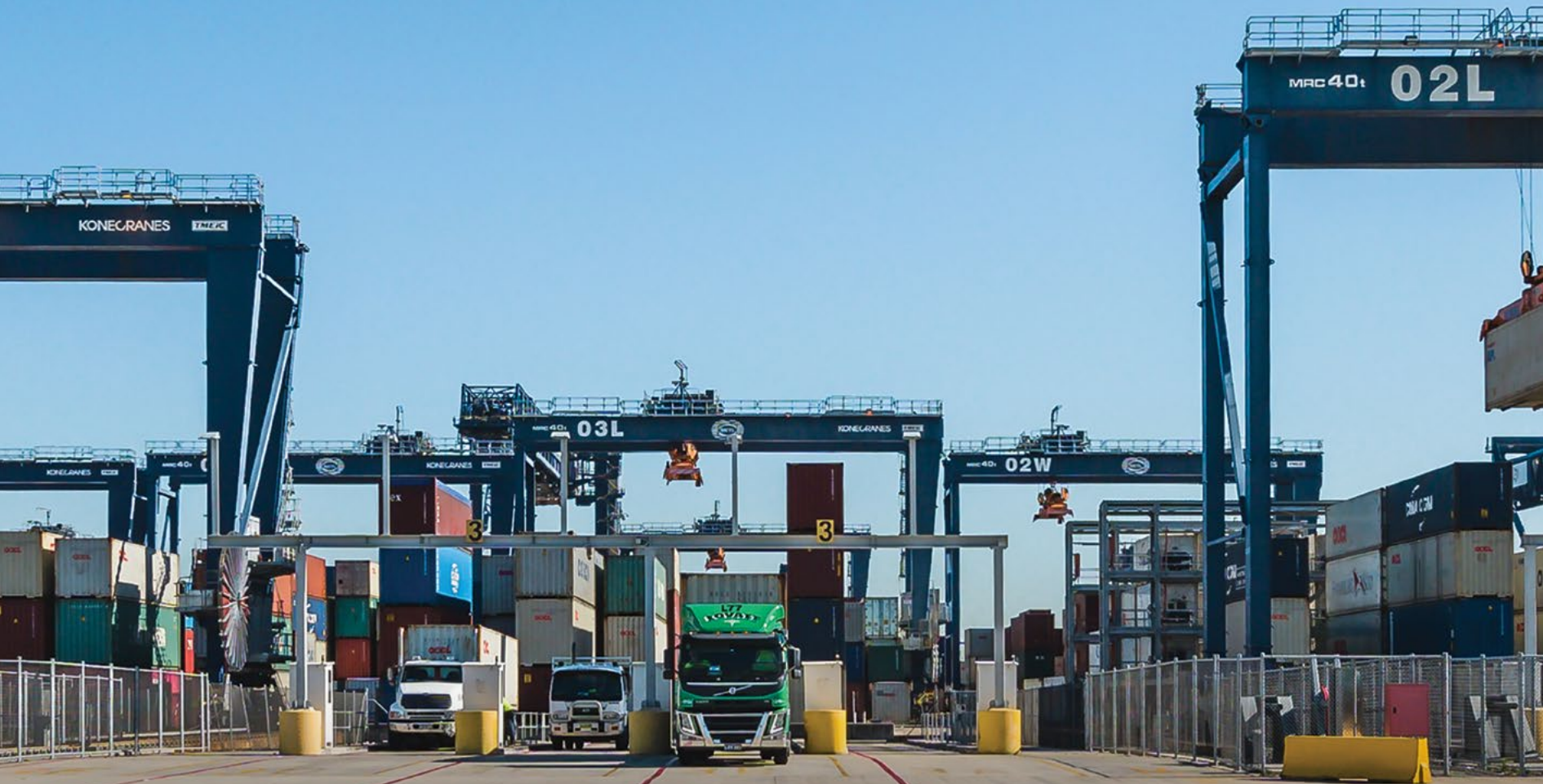
Trucks delivering and receiving containers through the Automated Stacking Cranes at Hutchison Ports Sydney (2019)
