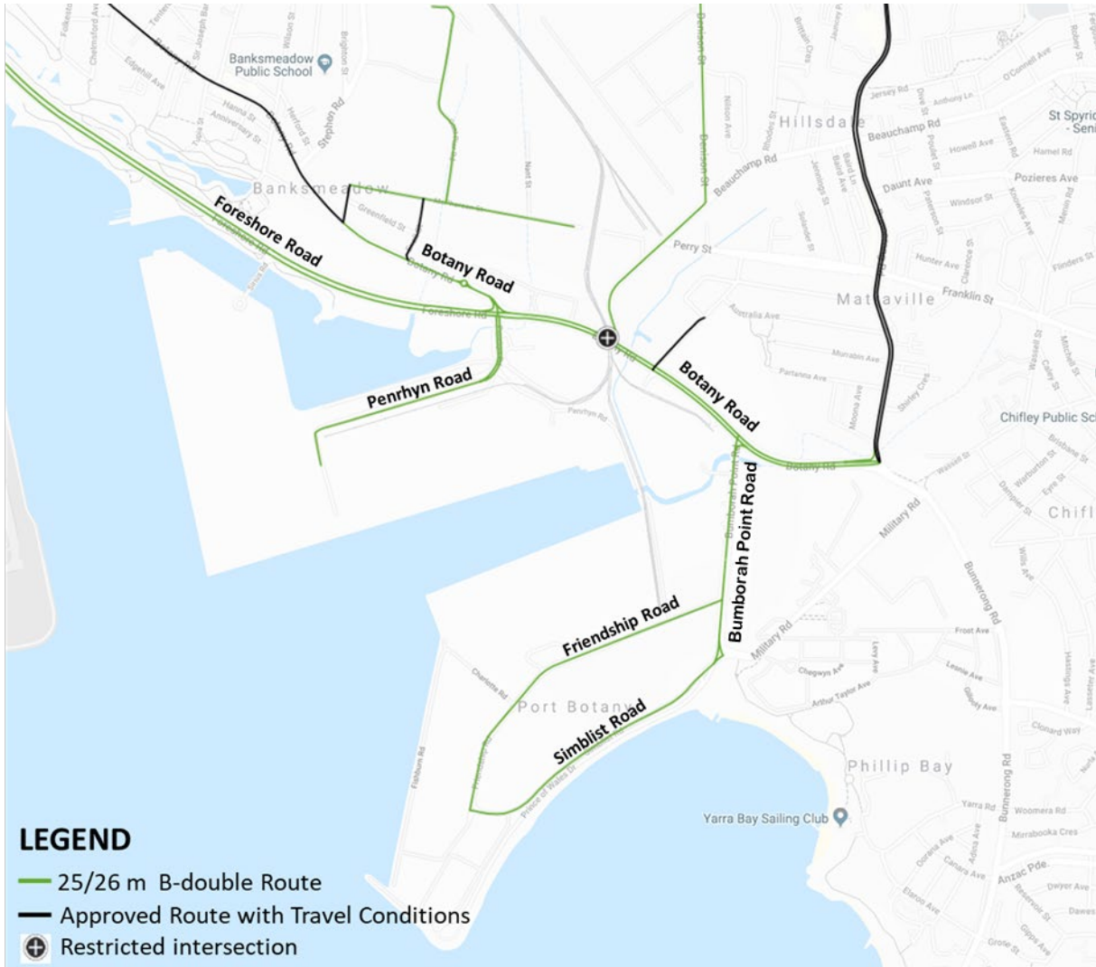
Figure 1. Access road network – 25/26 m B-double
