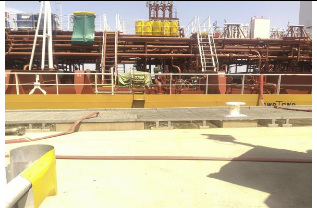
Hoses connected to the Stolt Renge for transfer of product
